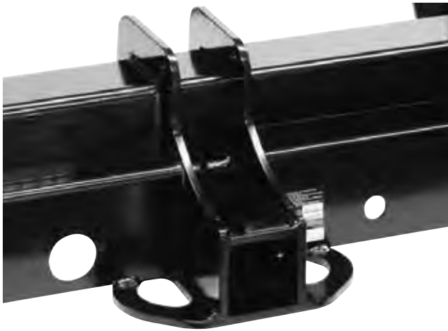
3-in Square Receiver Tube Opening
