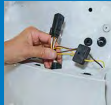
3. Route T-connector to the tail light harness.
