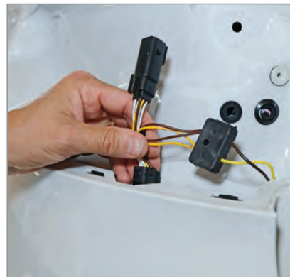
3. Route T-Connector to the tail light harness.
