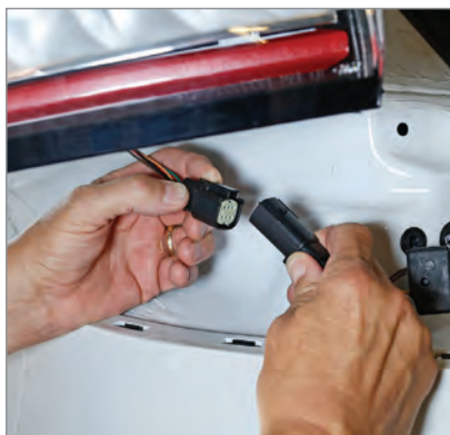
4. Plug the tail light into the T-Connector.
